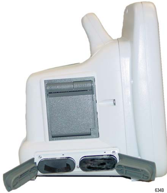
Monitor with Battery Packs
