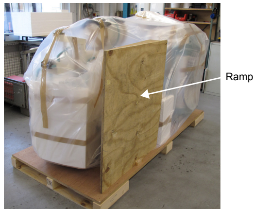
Fig. 13-19 Position of the ramp on the pallet
