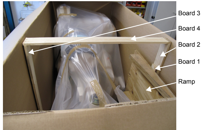
Fig. 13-20 Packing of the ramp
