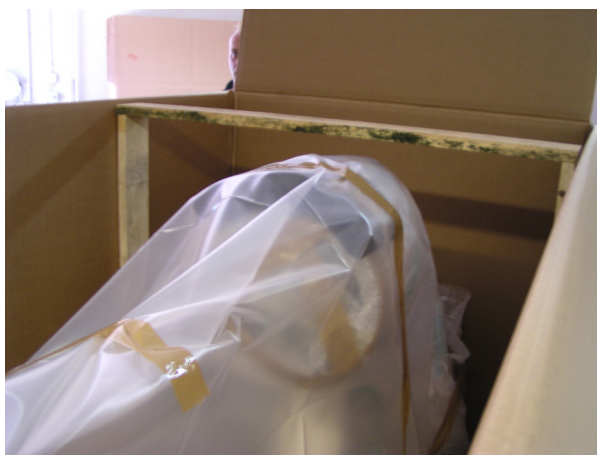
Fig. 3-2 Boards for cardboard box stabilization (USA)
