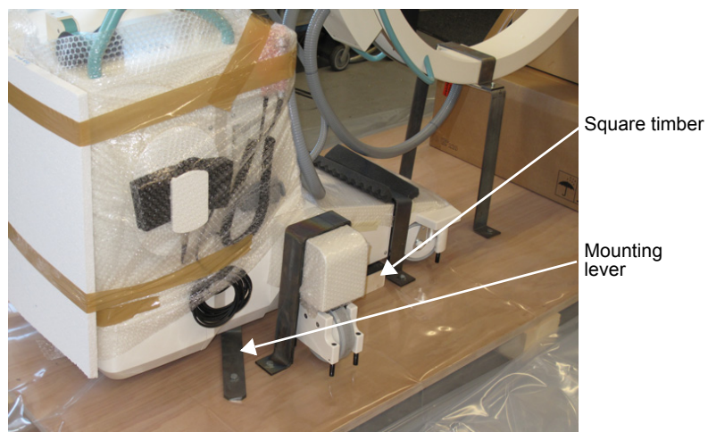
Fig. 13-7 C-arm stand with underlaid square timber and secured mounting lever.
