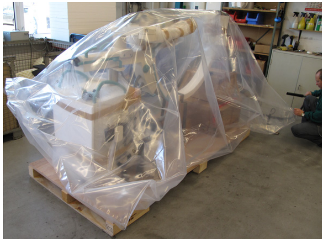
Fig. 13-22 Removing the air with suction
