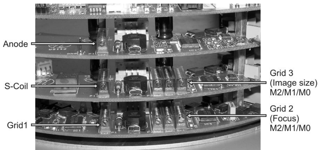
Fig. 6-2 U512, U513, U514 potentiometer location
