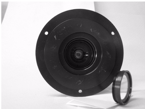
Fig. 6-9 Scattered light lens removed, lens removal tool
