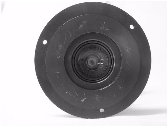
Fig. 6-8 Scattered light lens location
