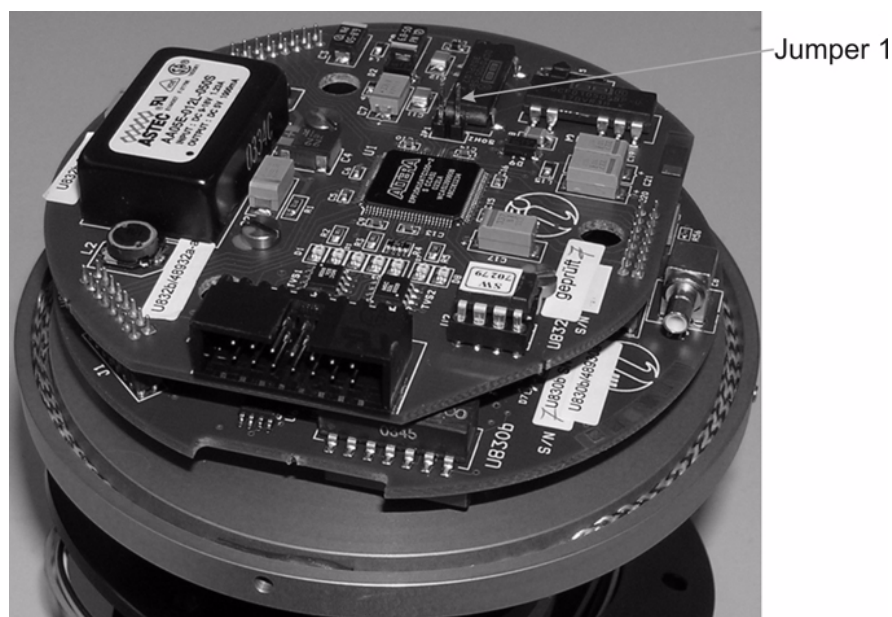
Fig. 6-13 Location of Jumper 1 on the CCD camera
